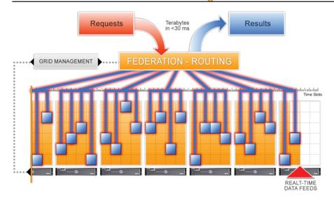
Psydex is designed around a shared-nothing, MPP architecture and easily scales using commodity hardware. Federators communicate with grid managers and index instances to intelligently route requests and aggregate, collate and fuse results.
